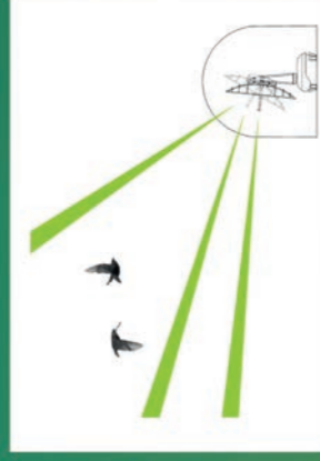
BirdScanMT1 - fixed-beam radar
